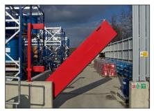
Gas-lift pivot barrier for vehicle access.
